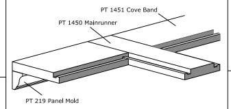
The mainrunners (and cross tees) that hit the wall are simply cut off at the wall to accommodate any size room. The cove band, which is machined on both ends with Key-lock joint, then snaps into and between the mains or cross tees.
