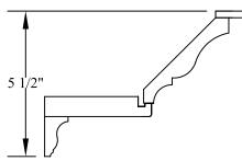
These pre-assembled drop-in panels create the coffered ceiling look. Available in 30" x 30" panels. Perimeter coffers are made to fit. Actual depth of coffer is 3-9/16". For clearance, allow 6" drop from joist to back of WOOD GRID®.
