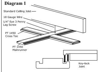
The **WOOD GRID®** Suspended Ceiling system hangs similar to metal grid except that it typically lays out on 30" or 32" centers when using the 3" grid. This layout is designed to accept our 28" x 28" medium coffers or 30" x 30" deep coffers. The patented Key-lock joint enables the cross tees to conveniently snap into the main runners. Screw eyes or metal T-bar brackets can be used with wire to suspend the grid.
