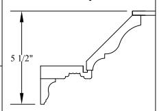
These pre-assembled drop-in panels create the coffered ceiling look. Available in 24" x 24" panels. Perimeter coffers are made to fit. Actual depth of coffer is 3-9/16". For clearance, allow 6" drop from joist to back of WOOD GRID®.
