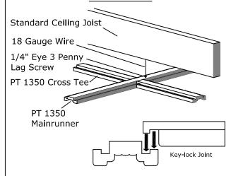
The **WOOD GRID®** Suspended Ceiling system hangs similar to metal grid except that it typically lays out on 30" or 32" centers when using the 3" grid. This layout is designed to accept our 28" x 28" medium coffers or 30" x 30" deep coffers. The patented Key-lock joint enables the cross tees to conveniently snap into the main runners. Screw eyes or metal T-bar brackets can be used with wire to suspend the grid.
